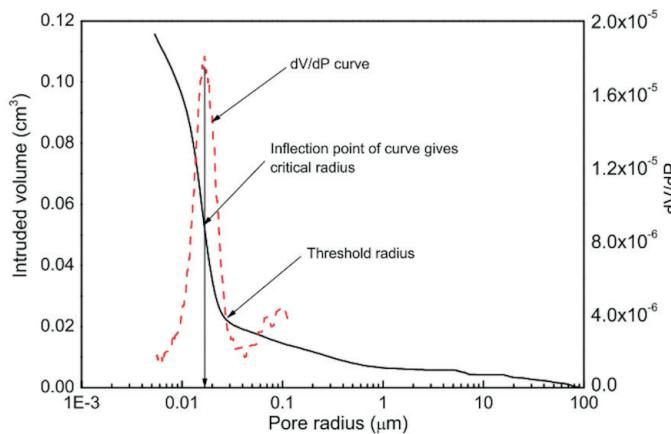
Fig. 4. Definition of critical and threshold pore radius [30]
