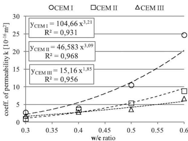
Fig. 8. Coefficient of permeability vs. w/c ratio [29]
