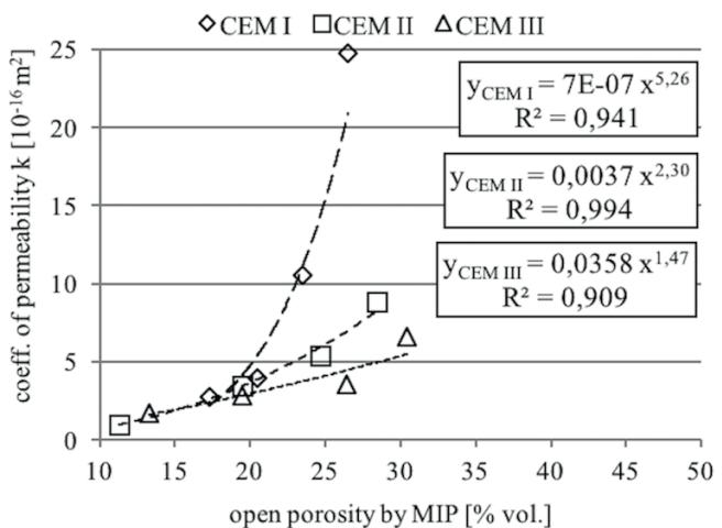
Fig. 10. Coefficient of permeability of cement paste vs. MIP porosity [29]
