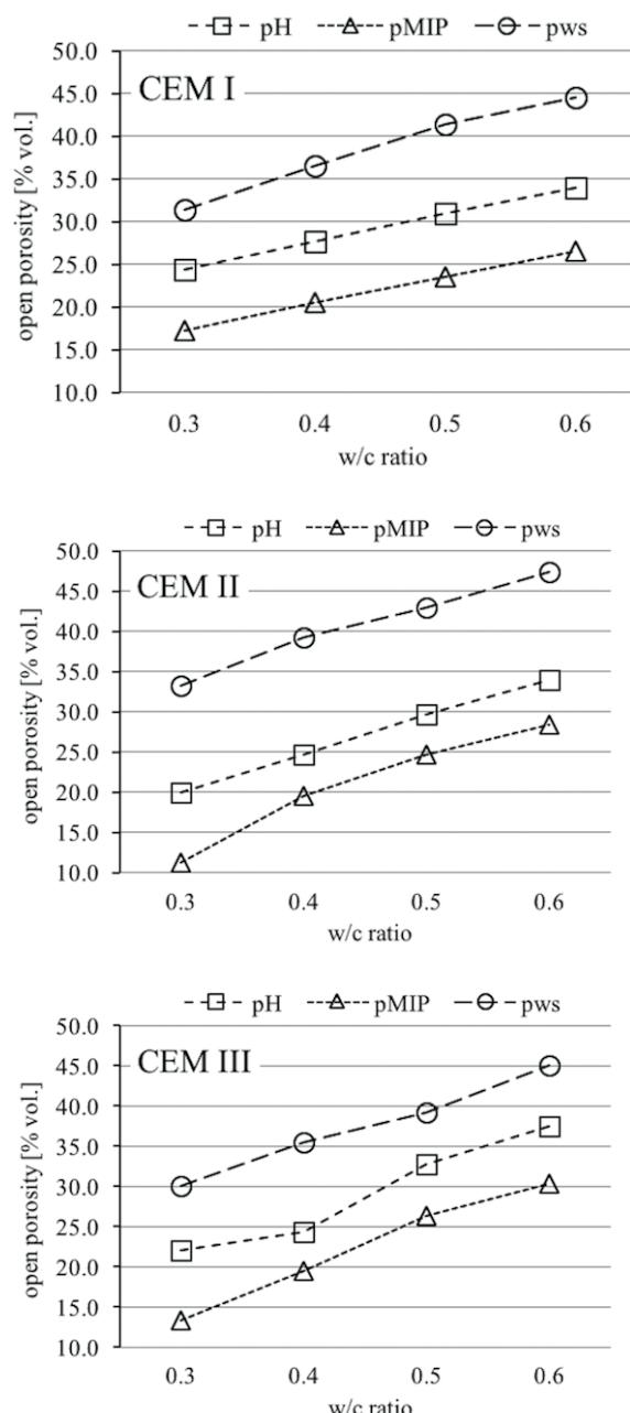
Fig. 2. The relationship between the helium porosity (pH), MIP porosity (pMIP), porosity determined based on water saturation (pWS) and the w/c ratio [29]
