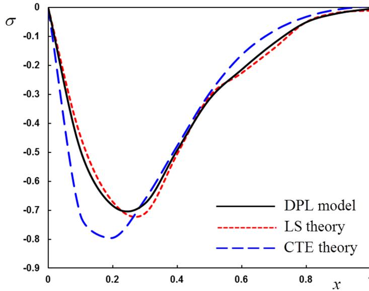
Figure 12: The thermal stress  $\sigma$  with distance  $x$  for different theories of thermoelasticity.
