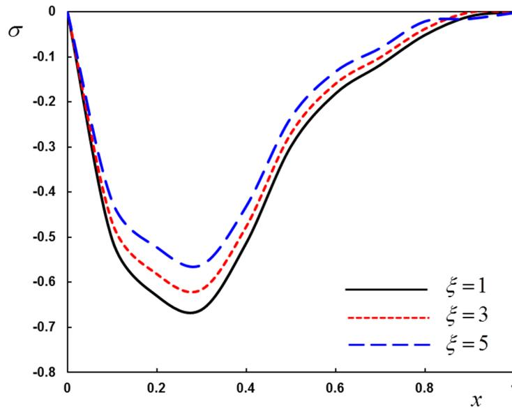
Figure 8: Dependence of the thermal stress  $\sigma$  on the laser intensity  $\xi$  along distance  $x$ .
