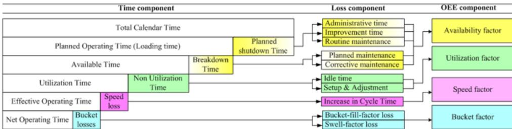
Fig. 4. OEE components of BELT equipment
