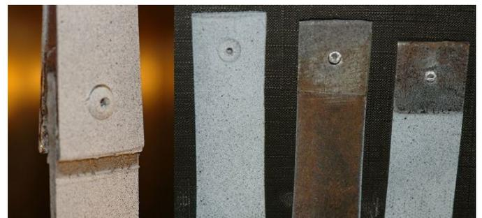
Fig. 3. Final failure of the adhesive-rivet joint
