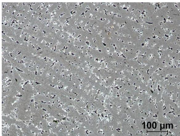
Fig. 4. Microstructure of homogenised Cu-3Ti alloy
