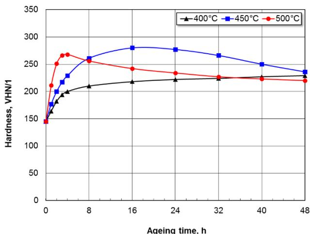
Fig. 10. Age hardening of hot rolled and cold drawn (85%) Cu-3Ti alloy
