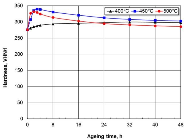
Fig. 13. Age hardening of hot rolled, solution treated and cold drawn (85%) Cu-3Ti alloy
