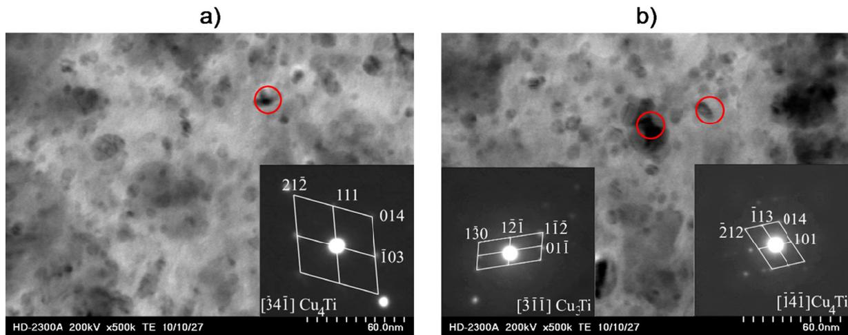
Fig. 16. Transmission electron micrographs (bright field and diffraction) of Cu-3Ti alloy hot rolled, solution treated, cold drawn (85%) and aged at 450°C for 1 h (a), 3 h (b)
