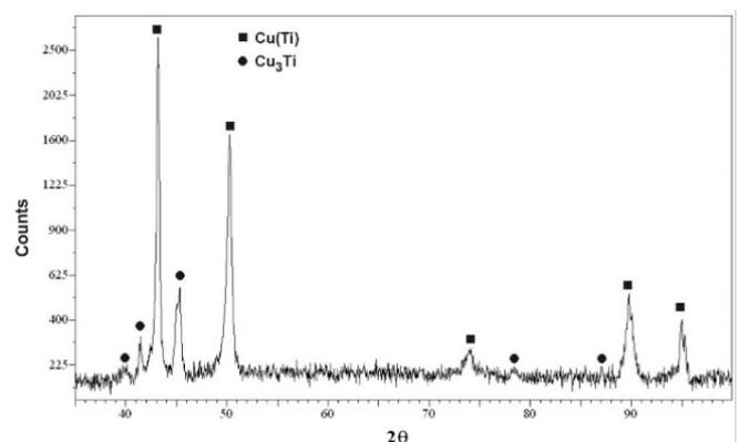
Fig. 3. XRD pattern of cast Cu-3Ti alloy
