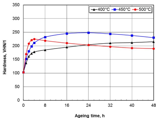
Fig. 6. Age hardening of cast Cu-3Ti alloy
