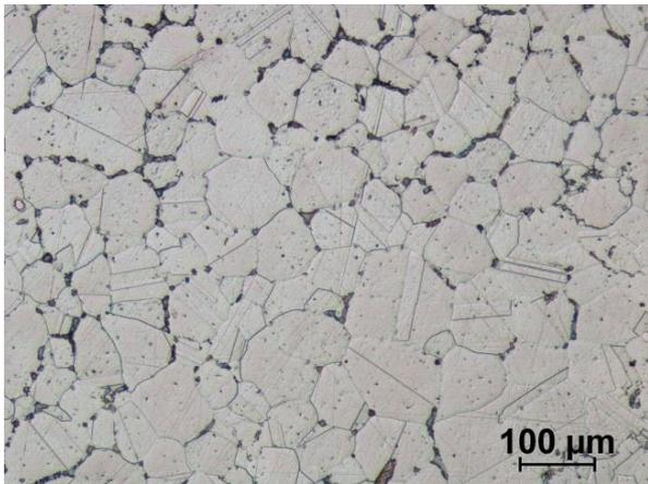
Fig. 9. Microstructure of hot rolled Cu-3Ti alloy
