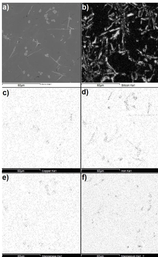
Fig. 9. Distribution of the most important elements in series: C, D, F and G on G-L example: a) SEM image of the structure and the distribution: b) Si, c) Cu, d) Fe, e) Mn, f) Mg; Magnification: 1200×
