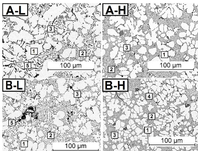
Fig. 6. Microstructures of castings A and B: 1 – phase  $\alpha$ , 2 – eutectic mixture, 3 – iron-rich phase, 4 – copper-rich phase, 5 – shrinkage-gas microporosity. Light microscope, magnification: 200 $\times$ , non-etched
