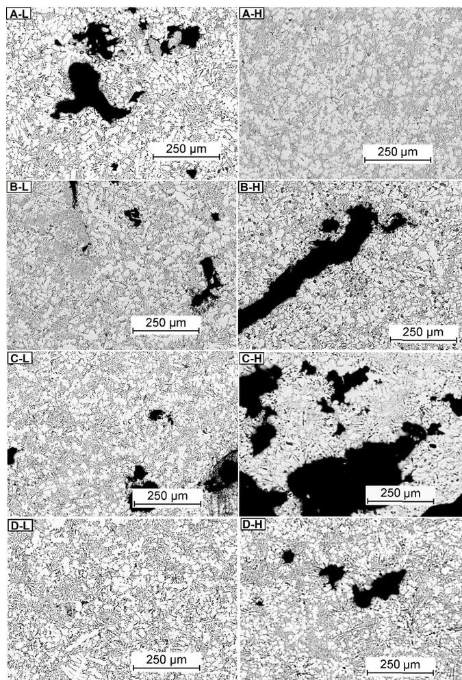
Fig. 3. View of samples' microstructure casts A-D, magnification: 50 $\times$ , non-etched
