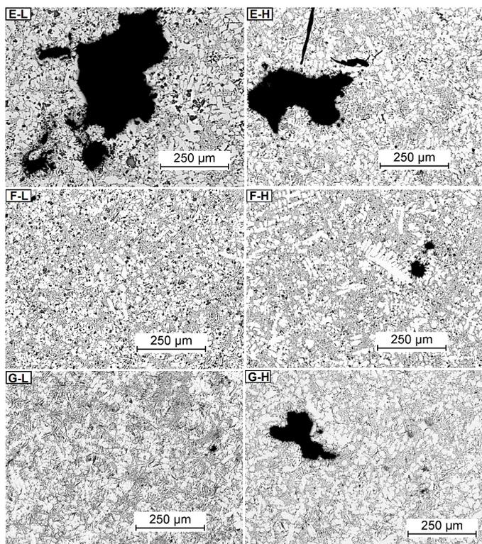
Fig. 4. View of samples' microstructure casts E-G, magnification: 50 $\times$ , non-etched
