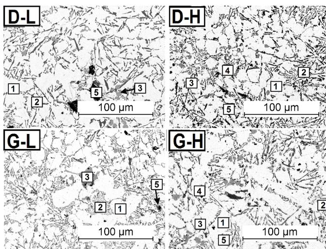
Fig. 7. Microstructures of castings D and G: 1 – phase  $\alpha$ , 2 – eutectic mixture, 3 – iron-rich phase, 4 – copper-rich phase, 5 – shrinkage-gas microporosity. Light microscope, magnification: 200 $\times$ , non-etched
