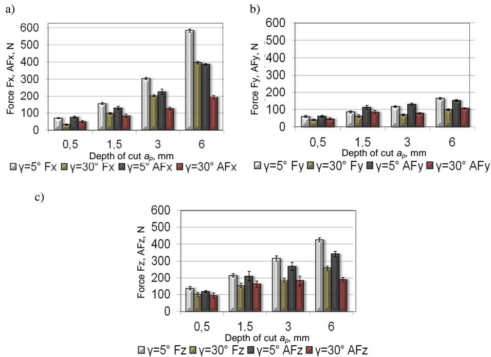
Fig. 5. The influence of change in depth of cut  $a_p$  (at  $f_z = 0.15$  mm/tooth) on cutting forces components and their amplitudes during milling of AZ91HP magnesium alloy: a)  $F_x$ ,  $AF_x$ , b)  $F_y$ ,  $AF_y$ , c)  $F_z$ ,  $AF_z$ ,  $f_z = 0.15$  mm/tooth,  $v_c = 800$  m/min
