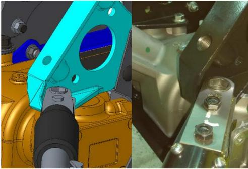
Fig. 11. Design modification and proper tooling selection as a solution for access issue.
