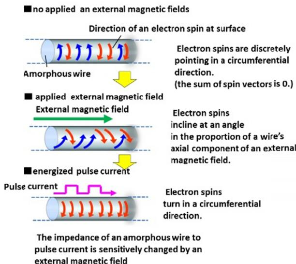
Fig. 4. Principle of external field detection in an amorphous wire
