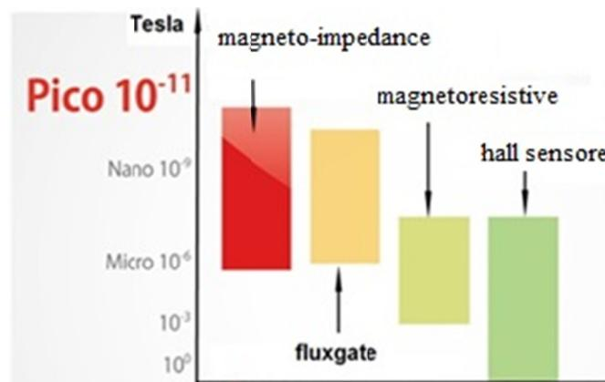
Fig. 2. Operating range of magnetic field sensors
