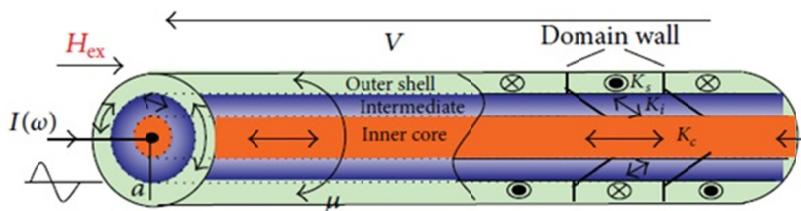
Fig. 5. Domain structure in an amorphous wire magnetised utilising the skin effect
