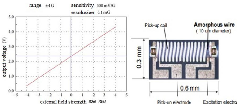
Fig. 7. Voltage vs field strength characteristic and a view of an MI sensor element (Mohri et al., 2015)
