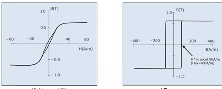
Fig. 3. Hysteresis loops of amorphous wires (<https://www.aichi-steel.co.jp/>)
