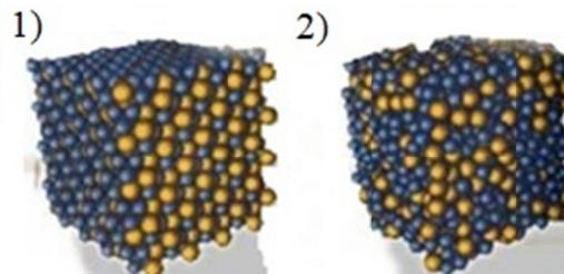
Fig. 1. Structure types 1) crystalline structure 2) amorphous structure (Dobrzański, 2006)
