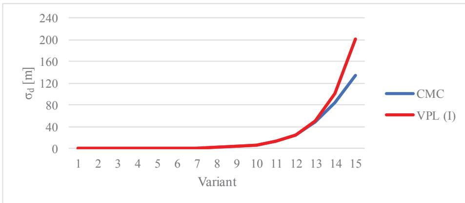
Fig. 3. Standard deviation of distance  $\sigma_d$  computed by VPL (I) and CMC estimate  $\hat{\sigma}_d$  for correlated coordinates ( $\rho_{X_A, Y_A} = 0.5$ ,  $\rho_{X_B, Y_B} = 0.5$ )
