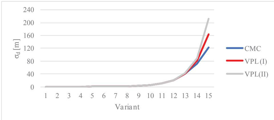
Fig. 2. Standard deviation of distance  $\sigma_d$  computed by VPL and CMC estimate  $\hat{\sigma}_d$  for uncorrelated coordinates
