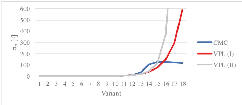
Fig. 4. Standard deviation of azimuth  $\sigma_A$  computed by VPL and CMC estimate  $\hat{\sigma}_A$  for uncorrelated coordinates
