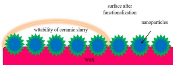
Fig. 5. Schematic diagram of functionalising of the wax pattern surface, used in the investment technology
