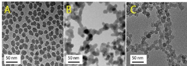
Fig. 4. Examples of TEM pictures of colloidal silica: A) dispersed, B and C) aggregated [8]
