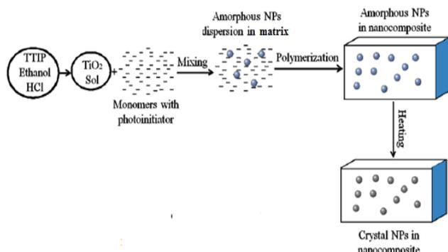
Fig. 1. Schematic of *in-situ* synthesis of hybrid materials [2]
