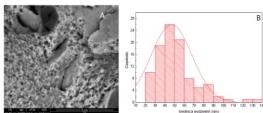
Fig. 8. Photo of the fracture of maraging steel with nanoprecipitates (a) and the distribution of precipitates diameters (b) [12]
