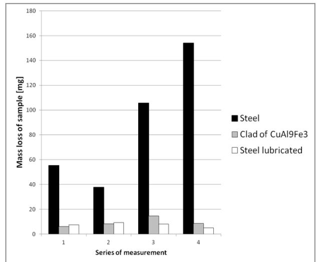
Fig. 8. The mass loss of tested samples after 200 revolutions, at the normal force 350 N
