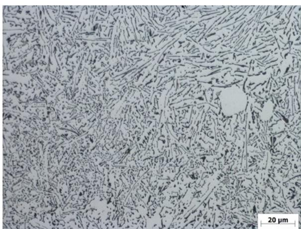
Fig. 5. Microstructure of samples, pressure 100 MPa, temperature 715°C, etched with 0.5% HF
