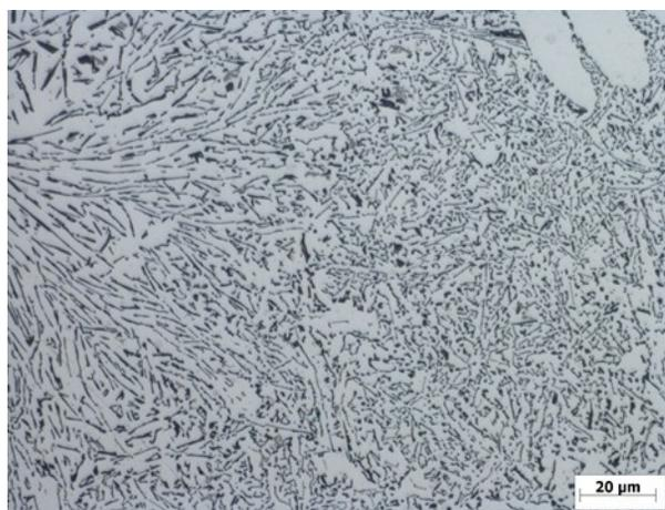
Fig. 7. Microstructure of samples, pressure 100 MPa, temperature 690°C, etched with 0.5% HF
