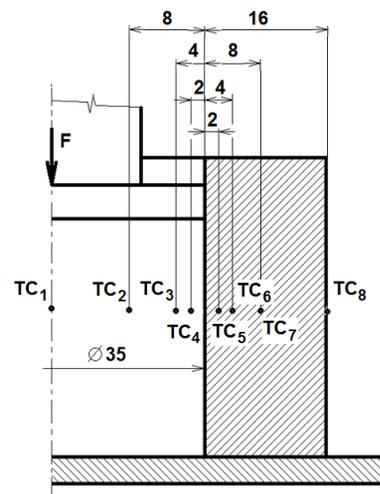
Fig. 1. Schematic drawing of measurement using thermocouples
