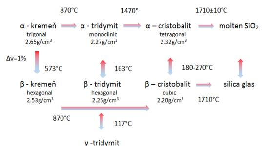
Fig. 3. Mechanism of polymorphic transformations  $\text{SiO}_2$
