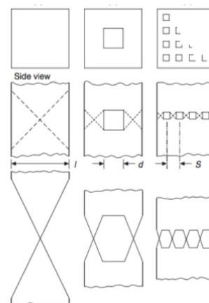
Fig. 7. Simple ductile failure model [2]
