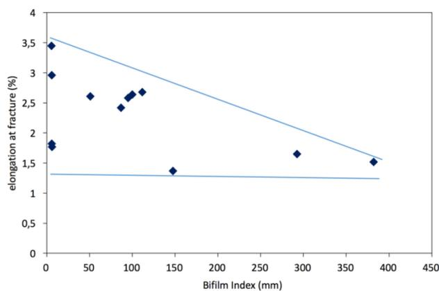
Fig. 6. The correlation between mechanical properties with bifilm index
