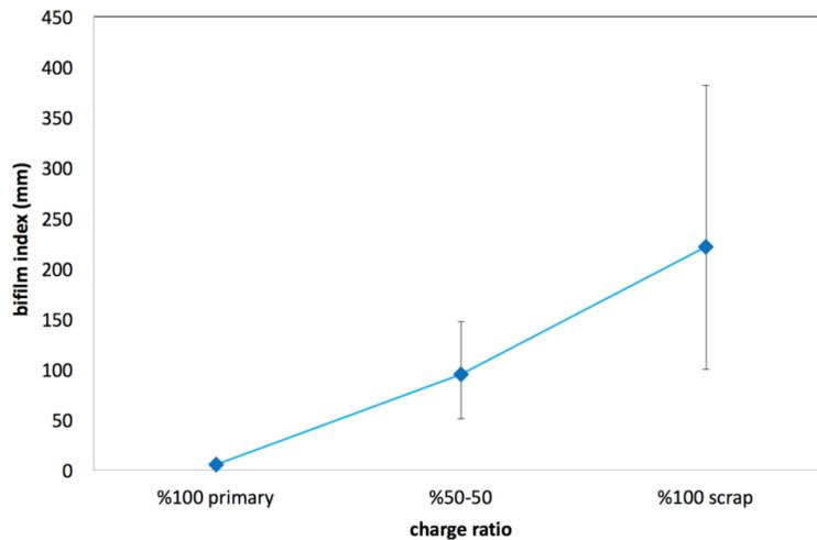
Fig. 4. Bifilm index of different charges
